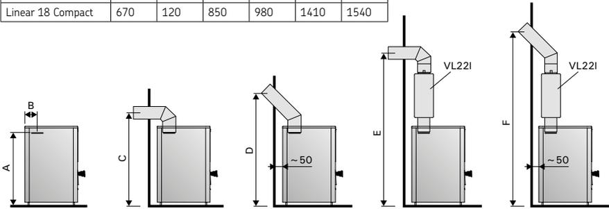
**EN: 9. Connecting the stove to a masonry flue via the rear connection opening**
