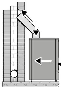
**EN: 11. Connecting the stove to a Harvia steel chimney**
