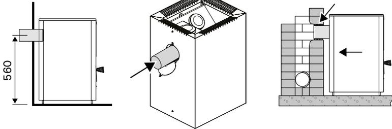
**EN: 10. Connecting the stove to a masonry flue via the upper connection opening**
